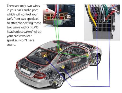
To enable the sound in your car's two rear speakers, you need to disconnect the two wires in the below picture, and order an extra speakers' adapter cable to connect the two wires with the two rear speakers of your car.
