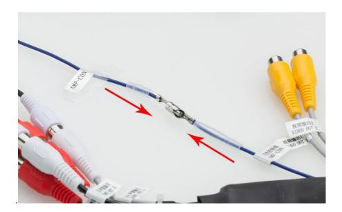
If your vehicle has no BOSE system, but it has the audio port as the picture shows, you need to make some modifications of the wires connection; otherwise, your rear amplified speakers will NOT have sound.
